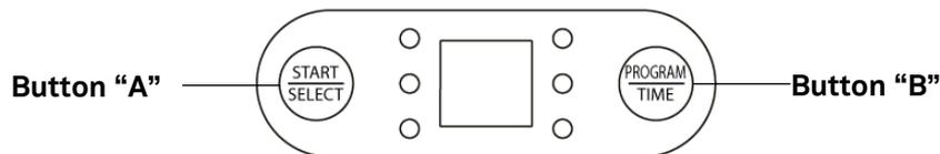
**Button A:** It has various functions that allow us to start up the unit and navigate through the 6 pre-established programs. It also has the unit stop function. Start function: One press allows the unit to start automatically on the first program.
